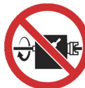
Any work piece stock extending the rear end of the headstock must be covered on its entire length. High danger of injury
