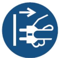
Make all machine adjustments or maintenance with the machine unplugged from the power source.
